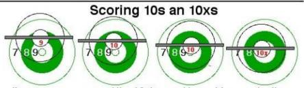
If you see any green of the 10 ring peeking out from under the edge of the gauge flange it is not a 10x.
